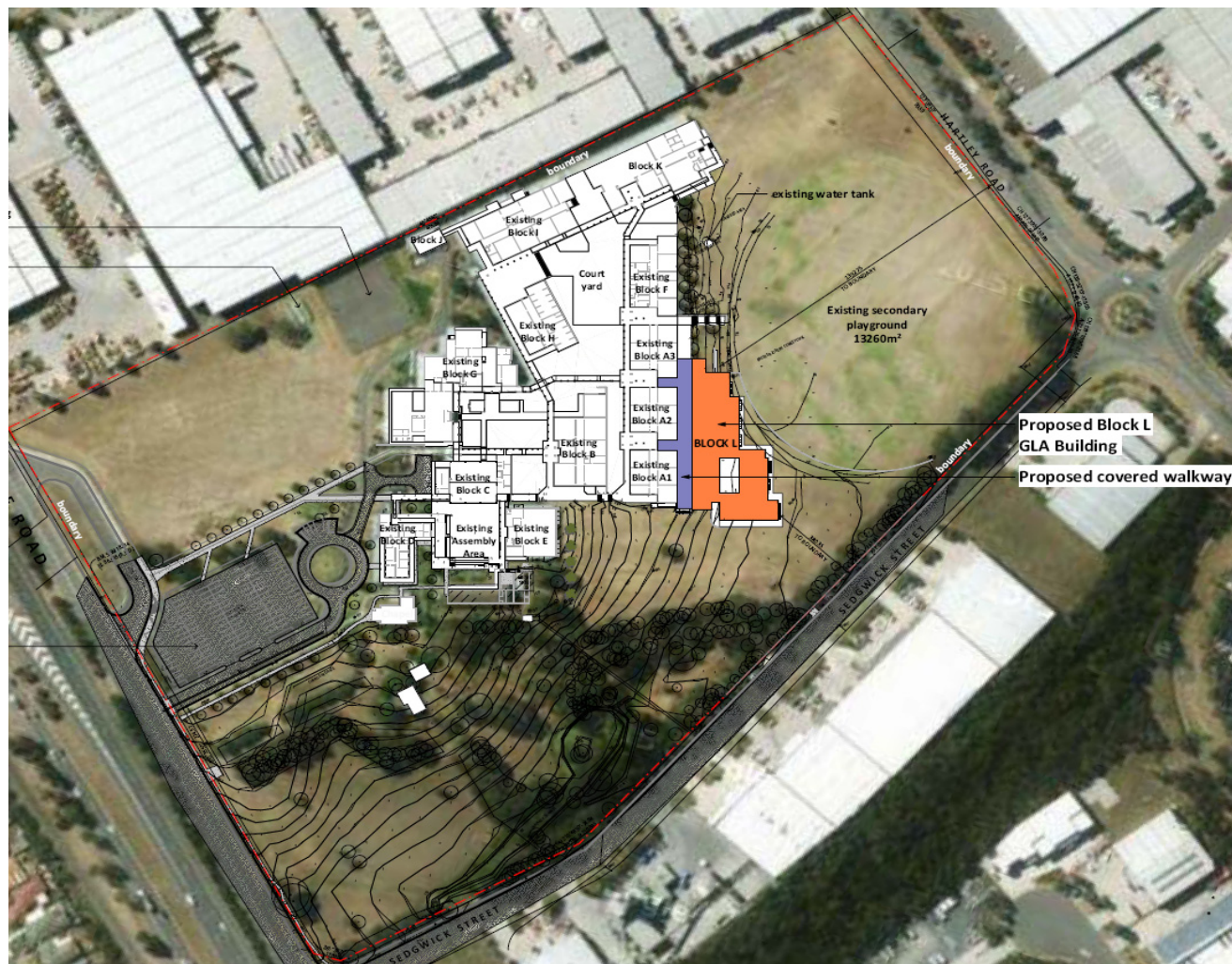
Figure 2 – Site Plan showing the location of the proposed Classroom extension.
